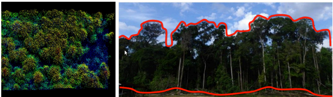
▲ Figure 04 – (a) LIDAR point cloud of a segment of the Amazon rainforest. (b) DSM and DTM to calculate the average height of a segment of forest.
