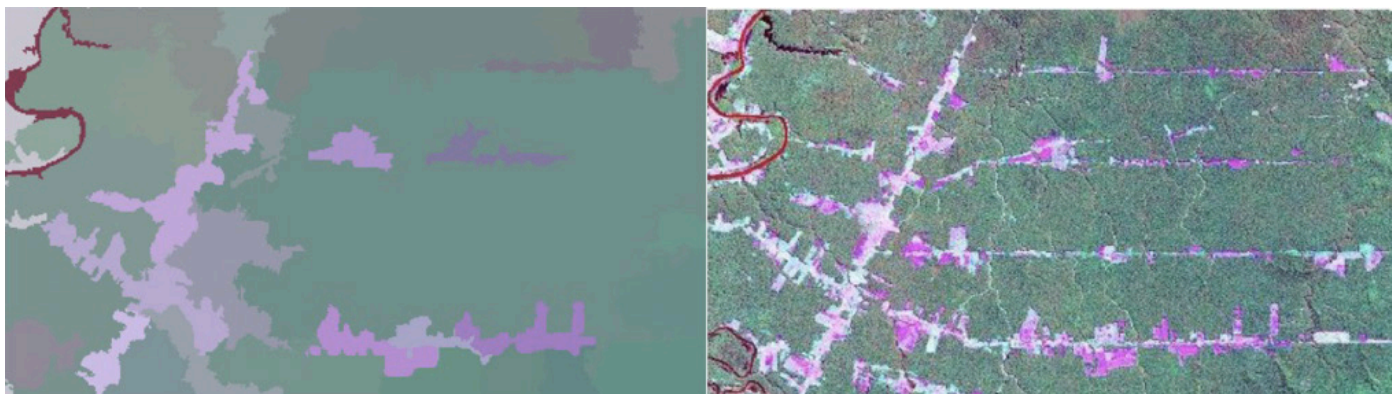
▲ Figure 06 – A satellite image example and its corresponding segmentation applying supervised ML (AI techniques).
