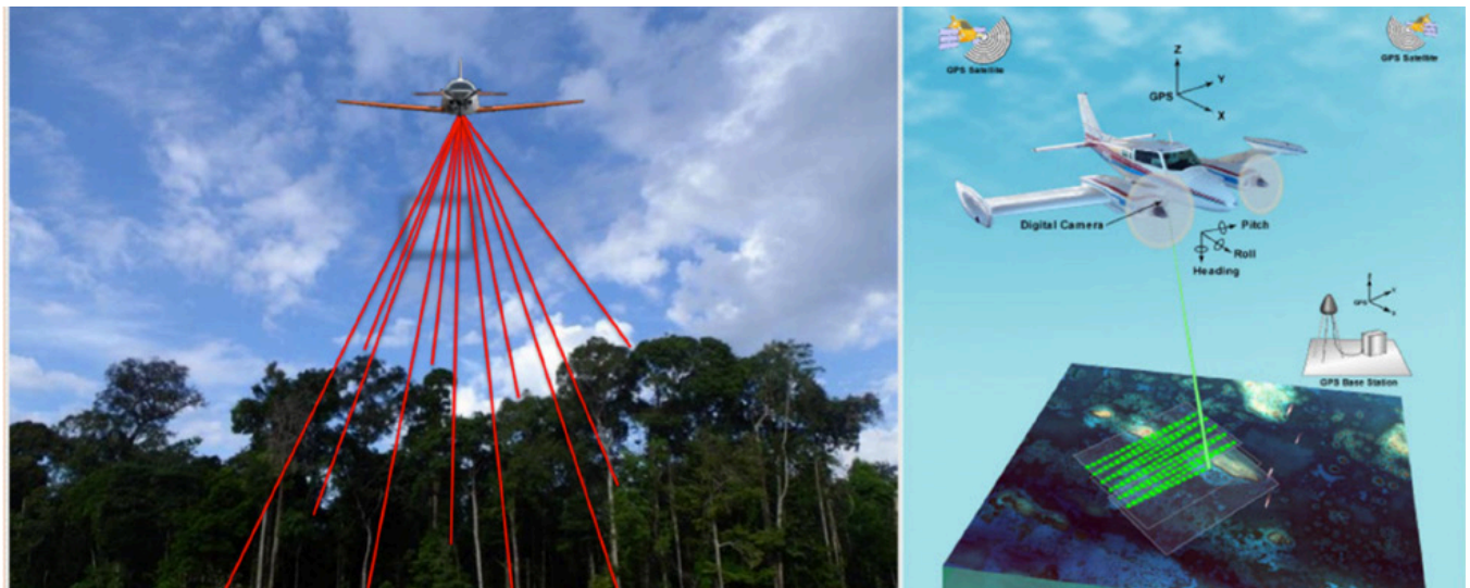
▲ Figure 03 – 3D high resolution remote sensing by LIDAR. Source: CADAF project.
