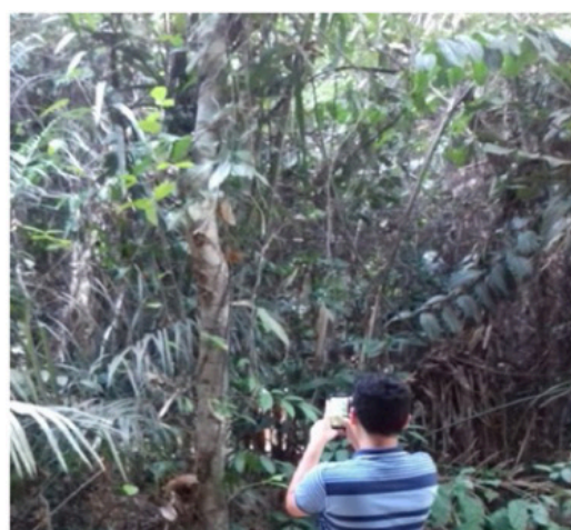
▲ Figure 02 – Tree-d Carb app - automatic determination of the DBH measure of a tree (Diameter at breast height) through the analysis of the photo from the camera of a rugged smartphone applying image processing and computational geometry techniques.
